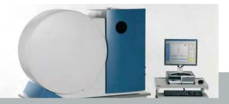
Additional SPECTRO ARCOS strengths include the new, extremely robust, free-running generator with a ceramic tube and solidstate power supply, the low maintenance and economical UV-PLUS system for high VUV transparency down to 130 nm, as well as the fast readout system with a dynamic range of eight decades and a transient measuring frequency of up to 10 Hz.
