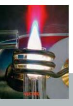
**Plasma Interface** Depending on the application, one of two different technologies is utilized to view the plasma. Axial plasma observation with the Optical Plasma Interface (OPI) is the right solution for the analysis of traces. Highest sensitivity and detection limits that are improved by up to a factor of 10 compared to radial observation are obtained with this method.
