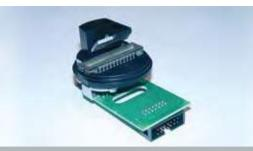
**Detector and Readout System** The SPECTRO ARCOS records the spectrum with 32 linear CCD detectors aligned to cover the entire wavelength range relevant to ICP-OES from 130 to 770 nm.
