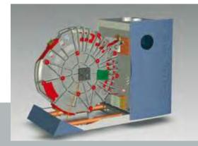
**UV-PLUS** The proven SPECTRO-UV-PLUS system is utilized in the SPECTRO ARCOS for measurements in the UV range. In this method, the optical system chamber is filled once with argon. The argon is circulated with a small membrane pump through a cleaning device; ensuring excellent long-term stability and eliminating disadvantages typical for systems with a vacuum or purge gas, such as contamination of the optical components.
